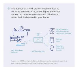
The Samsung SmartThings Water Leak Detector follows this pattern with a straightforward, easy-to-use app that alerts you if water is detected or if the humidity or temperature falls outside your preset levels, allowing you to personalize the alerts.
